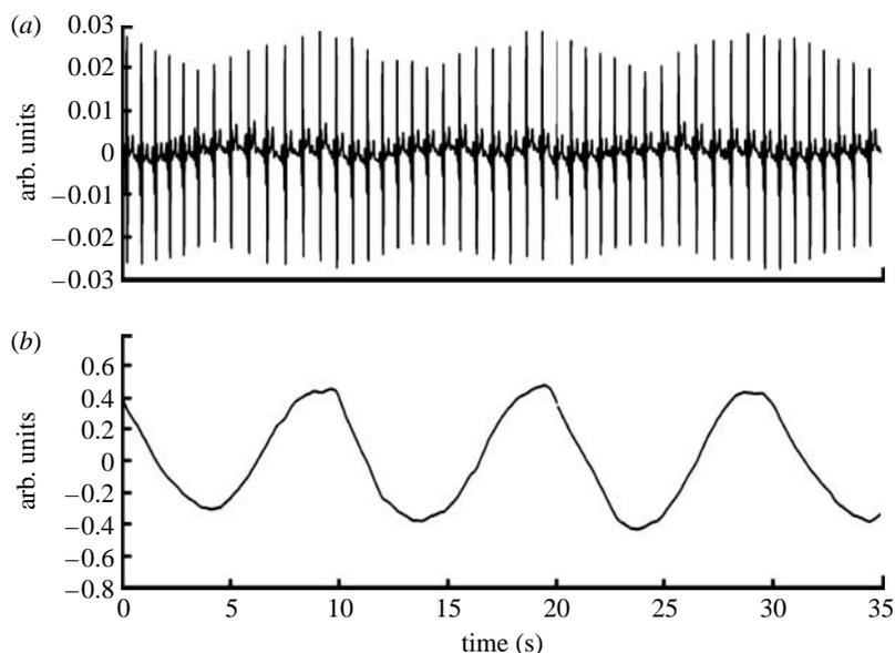
Figure 3. An example of the modulation of the ECG by respiration. (a) The ECG signal and (b) the simultaneously recorded chest respiratory effort signal. The modulation of the amplitude of the QRS wave by respiration is clearly seen.
