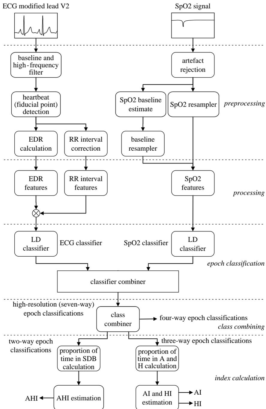
Figure 1. Simultaneous ECG and oximetry system for identifying epochs of apnoea and estimating AI, HI and AHI from overnight recordings.
